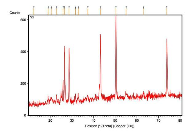
Figure: 1 Diffractogram of graphite and TiO<sub>2</sub> coated absorber.
