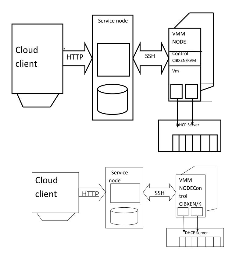
The virtual machine monitor of Nimbus is XEN and KVM the cluster are virtualized with the deployment of virtual machine.
