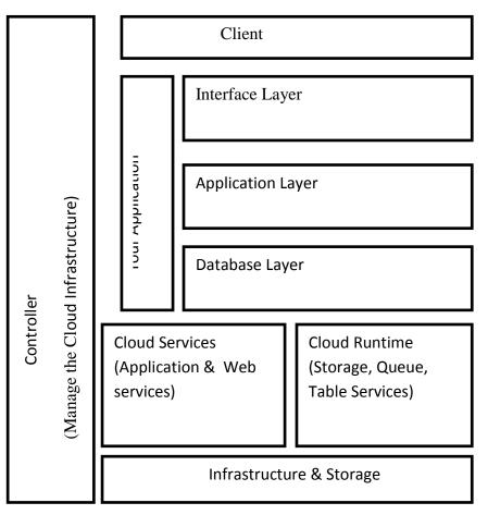
Cloud computing architecture refers to the various components and sub components of cloud that build the structured of the system. Broadly this architecture it can be classified into the frontend and the backend. The frontend and backend is connected to each other we are virtual network or the internet besides there are other components like middle ware cloud resources etc.
