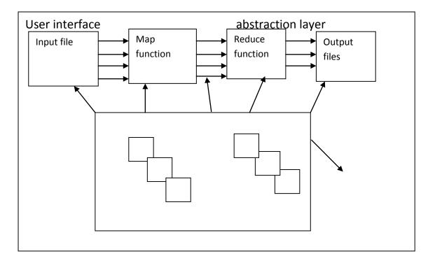
It is a software framework which supports parallel and distributed computing on large data sets. This software framework abstracts the dataflow of running a parallel program on a distributed computing system by providing users with two interfaces in the form of 2 functions.
